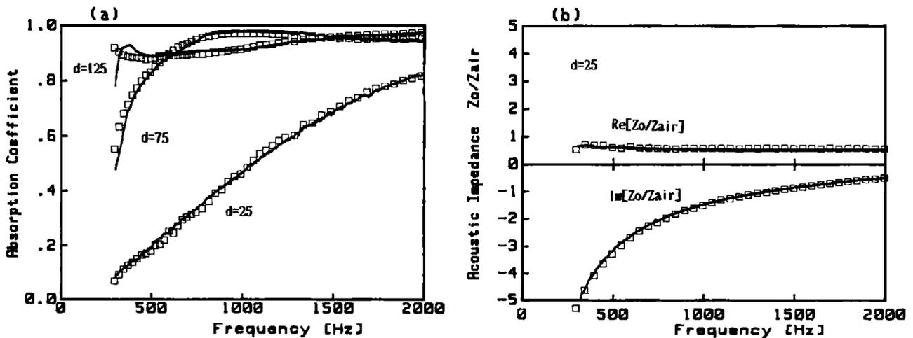
FIG. 7. (a) Comparison between calculated (—) and measured ( $\square$ ) normal absorption coefficient for 25-, 75-, and 125-mm-thick glass wool backed by a rigid wall; (b) comparison between calculated (—) and measured ( $\square$ ) normal acoustic impedance for 25-mm-thick glass wool backed by a rigid wall, where the calculation was based on the properties that were obtained at  $d = 50$  mm and  $(L, L') = (20, 70)$  mm.
