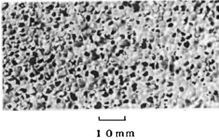
FIG. 2. Porous aluminum absorbing material.
