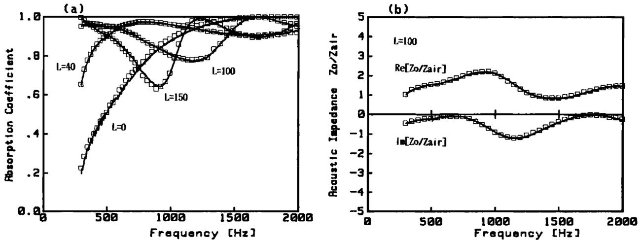
FIG. 6. (a) Comparison between calculated (—) and measured ( $\square$ ) normal absorption coefficient for 50-mm-thick glass wool with an air space depth of  $L = 0, 40, 100,$  and  $150$  mm; (b) comparison between calculated (—) and measured ( $\square$ ) normal acoustic impedance for 50-mm-thick glass wool with a 100-mm air space depth, where the calculation was based on the properties that were obtained at  $d = 50$  mm and  $(L, L') = (20, 70)$  mm.
