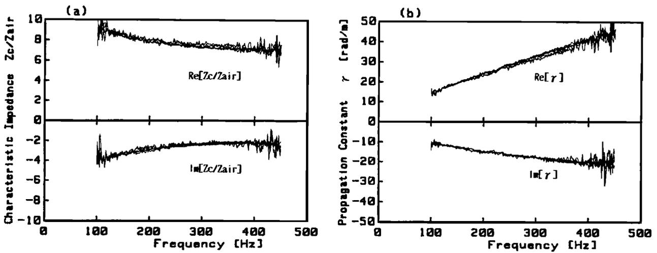
FIG. 5. (a) The characteristic impedance of porous aluminum normalized by air; (b) the propagation constant of porous aluminum, where both properties were obtained at  $d = 20$  mm and  $(L, L') = (20, 40)$  mm,  $(20, 70)$  mm,  $(20, 100)$  mm,  $(40, 70)$  mm, and  $(40, 100)$  mm.
