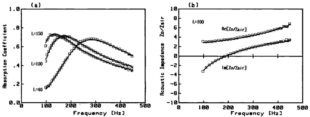
FIG. 8. (a) Comparison between calculated (—) and measured ( $\square$ ) normal absorption coefficient for 20-mm-thick porous aluminum with air space depths of  $L = 40, 100$ , and  $150$  mm; (b) comparison between calculated (—) and measured ( $\square$ ) normal acoustic impedance for 20-mm-thick porous aluminum with a 100-mm air space depth, where the calculation was based on the properties that were obtained at  $d = 20$  mm and  $(L, L') = (20$  mm,  $70$  mm).
