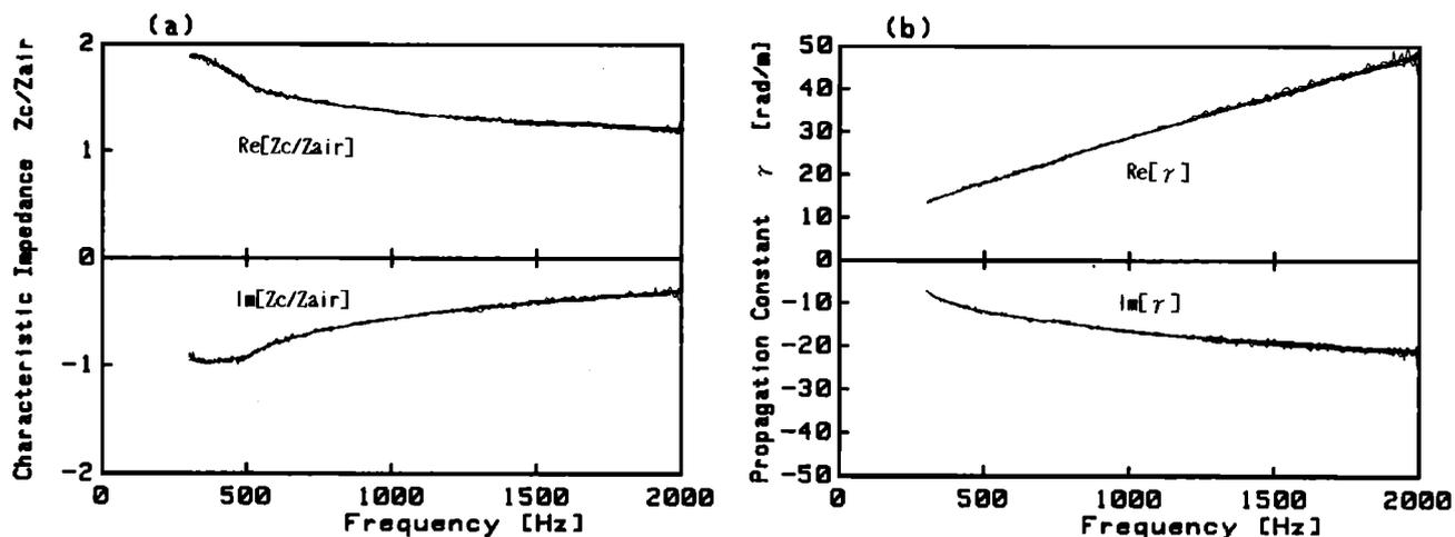
FIG. 3. (a) The characteristic impedance of glass wool normalized by air; (b) the propagation constant of glass wool, where both properties were obtained at  $d = 50$  mm and  $(L, L') = (20, 40)$ ,  $(20, 70)$ ,  $(20, 100)$ ,  $(40, 70)$ ,  $(40, 100)$ , and  $(70, 100)$ .
