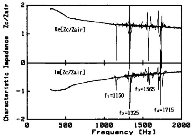
FIG. 4. The characteristic impedance of glass wool normalized by air, where it was obtained at  $d = 50$  mm and  $(L, L') = (20, 150)$ ,  $(20, 170)$ ,  $(40, 150)$ ,  $(40, 170)$ , and  $(70, 170)$ .
