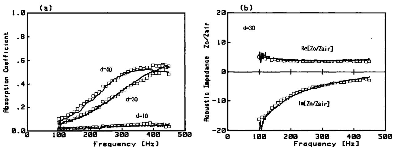
FIG. 9. (a) Comparison between calculated (—) and measured ( $\square$ ) normal absorption coefficient for 10-, 30-, and 40-mm-thick porous aluminum test materials backed by a rigid wall; (b) comparison between calculated (—) and measured ( $\square$ ) normal acoustic impedance for 30-mm-thick porous aluminum backed by a rigid wall, where the calculation was based on the properties that were obtained at  $d = 20$  mm and  $(L, L') = (20$  mm,  $70$  mm).
