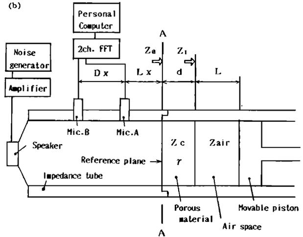
FIG. 1. (a) Experimental apparatus used to measure the characteristic impedance and propagation constant; (b) block diagram of the impedance tube and accessory equipment.
