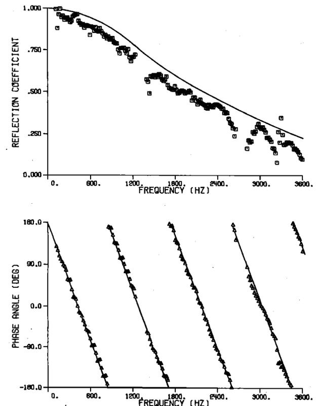
FIG. 7. Power reflection coefficient and phase angle for case II. Solid line: theory; open square, open triangle: experiment
