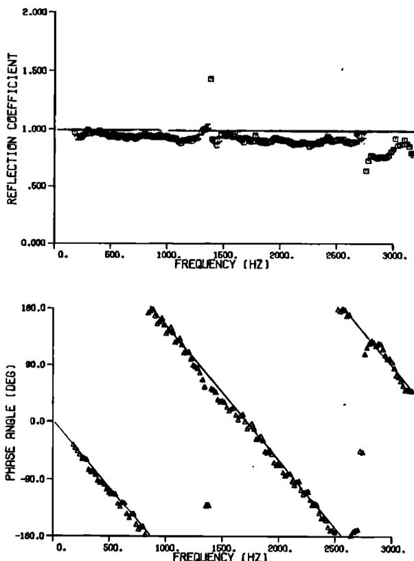
FIG. 5. Power reflection coefficient and phase angle for case I. Solid line: theory; open square, open triangle: experiment.
