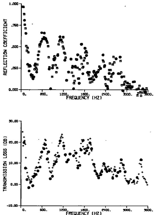
FIG. 9. Reflection coefficient and transmission loss for the prototype automotive muffler. Filled circle: SWR method; open square, plus sign: two-microphone random-excitation method.
