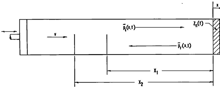
FIG. 1. Tube with unknown termination impedance  $Z_n(f)$  excited by randomly vibrating piston.
