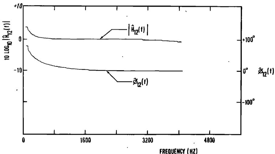
FIG. 4. Gain and phase shift between the two microphone/amplifier systems.
