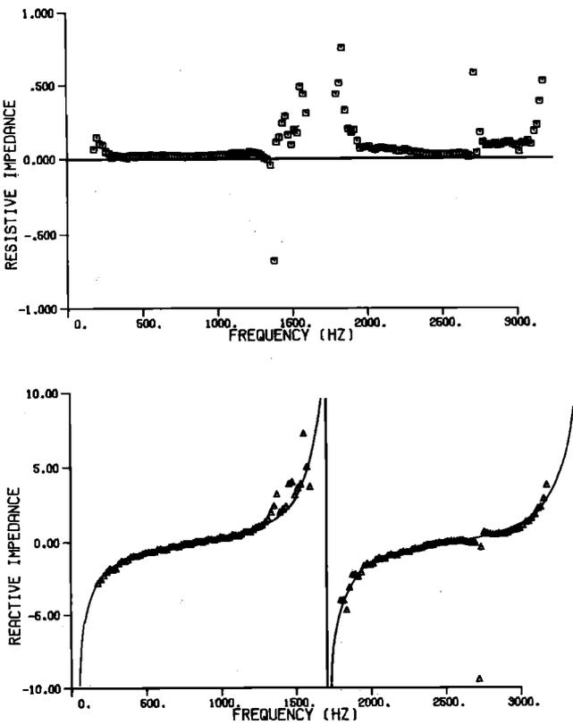
FIG. 6. Resistive and reactive impedance for case I. Solid line: theory; open square, open triangle: experiment.
