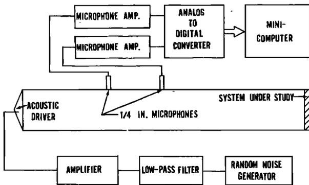
FIG. 3. Experimental set-up used in determination of impedance and power reflection coefficient using the two-microphone random-excitation method.
