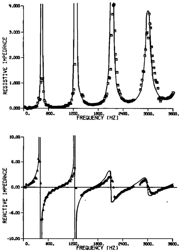
FIG. 8. Resistive and reactive impedance for case II, Solid line: theory; open square, open triangle: experiment.
